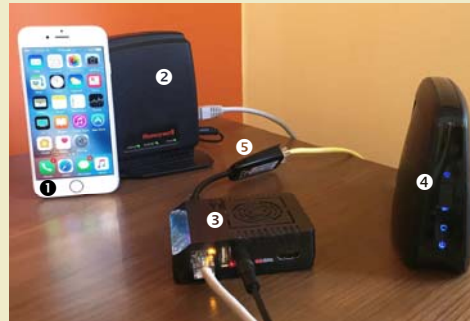
Figure 2: NetID and some supporting hardware. From left to right: ① an Apple iPhone 6™, ② a Honeywell RedLink™ Internet gateway, ③ an ODROID-XU4™ platform (hosting the NetID software), and ④ a Linksys™ WAP610N 802.11n Access Point. The ODROID™ has two gigabit Ethernet connections, one onboard and the other via a ⑤ Linksys™ USB3g1g USB-to-Ethernet dongle, enabling it to be in-line with the network's Internet connection, similar to a user's home router.
