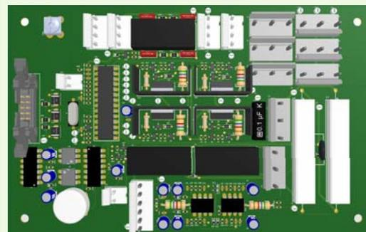
Figure 3 (left): The same optimized GLCI box PCB modeled in 3D. The 3D footprints to each component are shown on this board, demonstrating how the PCB will look when constructed.
