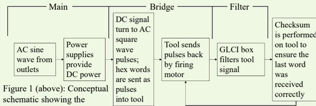
Figure 1 (above): Conceptual schematic showing the functions of the PCB.
