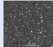
Figure 1: Image of the 3.0 at% Si sample obtained by SEM.
