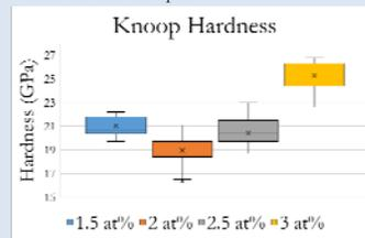
Graph 1: The graph to the left represents the distribution of hardness values for the 15 indents measured for each sample.
