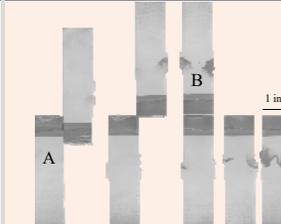
Figure 4: A sample that displays (A) cohesive failure and (B) adhesive failure.
