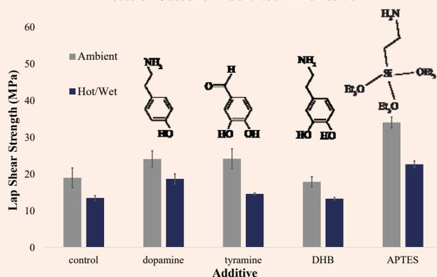
Graph 1: Comparison of adhesive performance of formulations with additives to the formulations without additive (e.g. control) and the industrial surface standard (APTES). Included are standard deviation error bars from a sample size of 10 coupons per condition.
