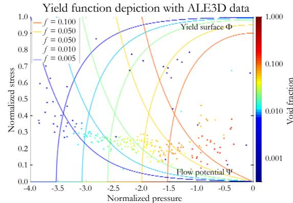
Graph 2 (above): Effective stress with pressure as a function of void fraction. The color of the curve or data point indicates the void fraction of the material with a value of 1 being entirely void, and a value of 0 having no void. The black line running through the middle is the predicted intersection point for the equations. It is at  $1 - \sqrt{2}$ .
