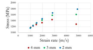
Graph 3 (left): The peak stress as a function of peak strain rate at various time steps. A positive correlation indicates that the material has begun spalling, while a negative correlation indicates that the material has resisted failure. Only the 4 mm simulation indicates time states after the wave reaches the free surface with no failure.
