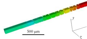
The failure patterns for each specimen were similar across simulations. There was one location which had only incipient spall in the 4 mm and 3 mm samples but exhibited complete spall in the 2 mm sample.
