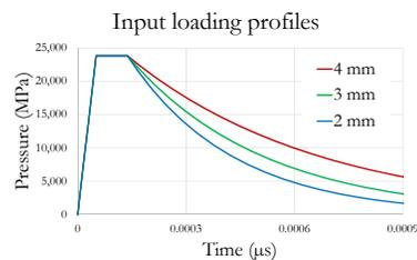
Graph 1 (above): The three primary pressure loading profiles used in the simulations.
