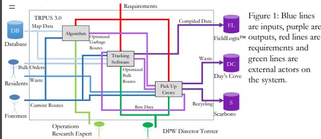
Figure 1: Blue lines are inputs, purple are outputs, red lines are requirements and green lines are external actors on the system.
