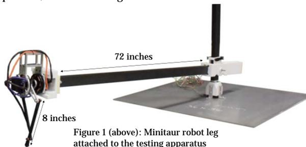
Figure 1 (above): Minitaur robot leg attached to the testing apparatus
