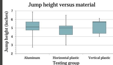
Graph 2 (left): Box-and-whisker plot of leg material versus jump height.
