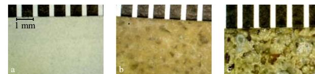
Figure 3 (above): Pictures of the same type of concrete before exposure (a), and after exposure to NH<sub>4</sub>NO<sub>3</sub> (b) and NH<sub>4</sub>Ac (c). Each was taken with a ruler of scale 1 mm.
