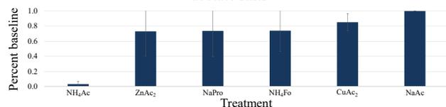
Graph 2 (above): Shows the load bearing capacity and standard deviation of concrete samples ( $N = 24$ ) after exposure to various acetate salts. The loads are reported as a percent of baseline for that concrete, so all the tests can be represented on the same scale.
