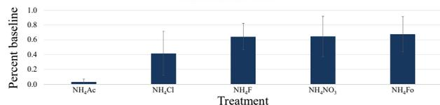
Graph 1 (above): Shows the load bearing capacity and standard deviation of concrete samples ( $N = 20$ ) after exposure to various ammonium salts. The loads are reported as a percent of baseline for that concrete, so all the tests can be represented on the same scale.
