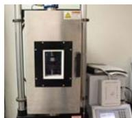
Figure 2 (right): The Universal Testing machine used to test each cube after exposure.
