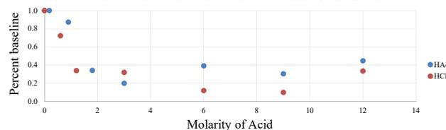
Graph 3 (above): Shows the load bearing capacity of concrete samples ( $N = 35$ ) after exposure to various molarities of hydrochloric and acetic acid. Points are averages of multiple tests ( $n = 2$  to 4), which is why there are less points than total samples.
