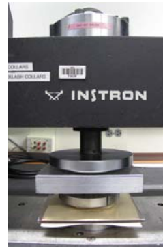
Figure 2 (left, bottom): Modified Bayer Taber® tester used to induce abrasion damage upon the glass specimen by oscillating laterally with the specimen secured in it.
