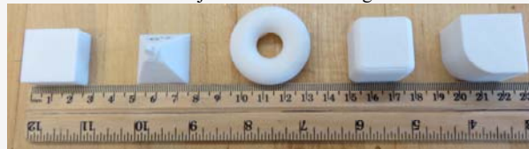
Figure 1. Printed test objects from left to right: Rectangle, Pyramid, Torus, Filleted Cube, Curved Corner
