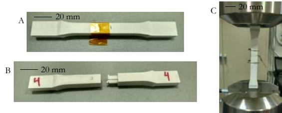
Figure 1: (A) SS sample before testing, (B) SS sample after testing, (C) SS sample in INSTRON™ tensile tester machine.
