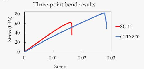
Graph 2: The average calculated stress and strain from the three-point bend test of 4 samples of each composite displays the flexural strength.
