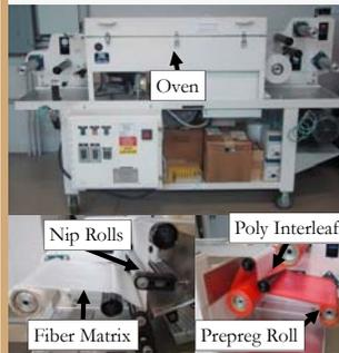
Figure 1 (top): Lab prepreg machine.
