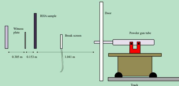
Figure 1 (above): Side view of experimental set-up.
