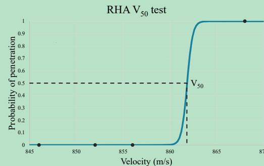
Graph 1 (above): The line graph above contains the five points collected from different trials with RHA. This was created for a baseline as comparison to test other compounds, especially FeMnAl. The  $V_{50}$  value is found at 861.8 m/s.
