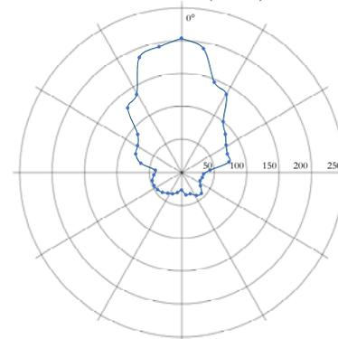
Graph 3 (left): Shows the distance of consistent reception with the receiver turned to various angles and the LED pointed directly at the receiver. While the shape of the graph is similar to the expected shapes, minute differences in angle and vertical angle and height of the transmitter are likely responsible for the irregular shape of the graph, instead of the smoother curve that would have been expected.
