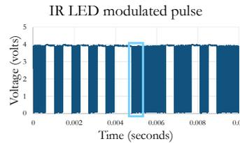
Graph 1 (left): Shows part of the modulated square wave that the IR LED pulses to transmit the identifier. Each bit is actually a series of 38 kHz pulses that is decoded by the receiver as a square wave shaped like the modulated pulse. The light blue box shows a close up of the pulse in Graph 2.
