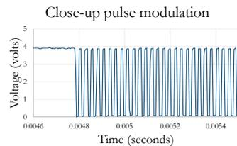
Graph 2 (left): Close-up view of the modulated pulses in the box in Graph 1. It can be seen that each modulated bit consists of a series of 38 kHz pulses that the receiver will read as a regular square wave.
